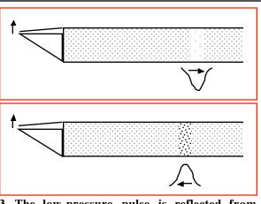
3. The low-pressure pulse is reflected from this closed end of the instrument and moves back to the other end. When it reaches the higher, normal air pressure, it largely reflects again, this time as a highpressure pulse.
