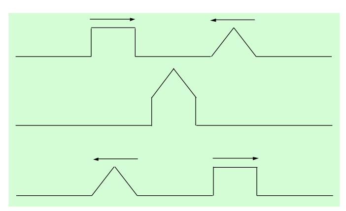
Figure 1.8: Wave superposition. Note in the middle drawing that the wave shape is simply the arithmetic sum of the amplitudes of each wave. Note also in the bottom drawing that the two waves have the same shape and amplitude as they had before encountering each other.
