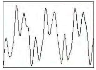
Figure The complicated 3.4: waveform shown here is typical of that produced by a musical instrument. This waveform can be produced by combining the waveform of the with fundamental frequency waveforms frequencies that having are integer multiples of the fundamental frequency.
