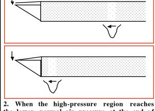
the lower, normal air pressure at the end of the instrument it is largely reflected. This causes the reflected pulse to be a negative or low-pressure pulse and has the effect of pulling the reed toward the body of the instrument, closing the gap sharply.
