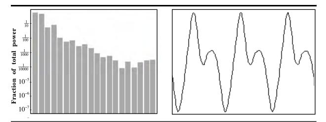
Figure 3.9:  $B_4$  played on the <u>BASSOON</u>. The power spectrum is much different for this high note played on the same bassoon. Over two octaves higher than the note producing the power spectrum in Figure 3.8, the first two harmonics dominate, producing almost all the power. The third and fourth harmonics produce far less than 10% of the total power and all the remaining higher harmonics produce less than 1% combined. The result is a simple waveform with an almost flute-like sound.
