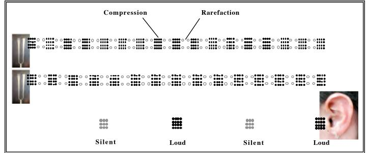
Figure 3.12: Beats. The two tuning forks have slightly different frequencies. This causes the sound waves produced by each one to interfere both constructively and destructively at various points. The constructive interference causes a rise in the intensity of the sound and the destructive interference causes silence. This pattern is repeated over and over causing the phenomenon of beats.
