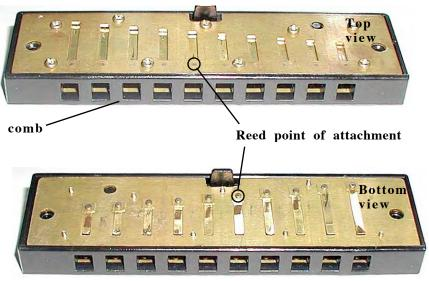
the mechanism is for the production of sound from the harmonica?
