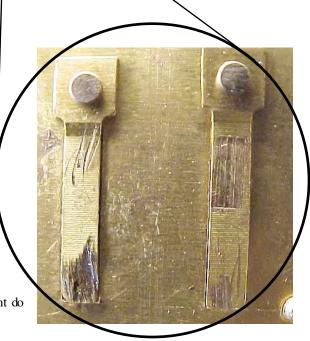
b. What does filing the reed near the point of attachment do to the frequency of the reed when it is vibrating?
