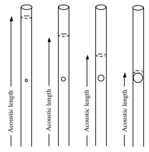
Figure 6.14: A hole drilled on the side of a pipe changes the acoustic length of the pipe. The larger the hole, the closer the acoustic length will be to the hole position.
