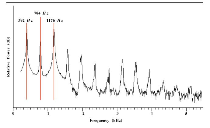
Figure 3.1: The "sound spectrum" of a flute shows the frequencies present when the G4 note is played. The first designated peak is the desired frequency of 392 Hz (the "fundamental frequency"). The next two designated peaks are the first and second "overtones." Since these and all higher overtones are integer multiples of the fundamental frequency, they are "harmonic." (Used with permission. This and other sound spectra can be found at http://www.phys.unsw.edu.au/music/flute/modernB/G4.html)
